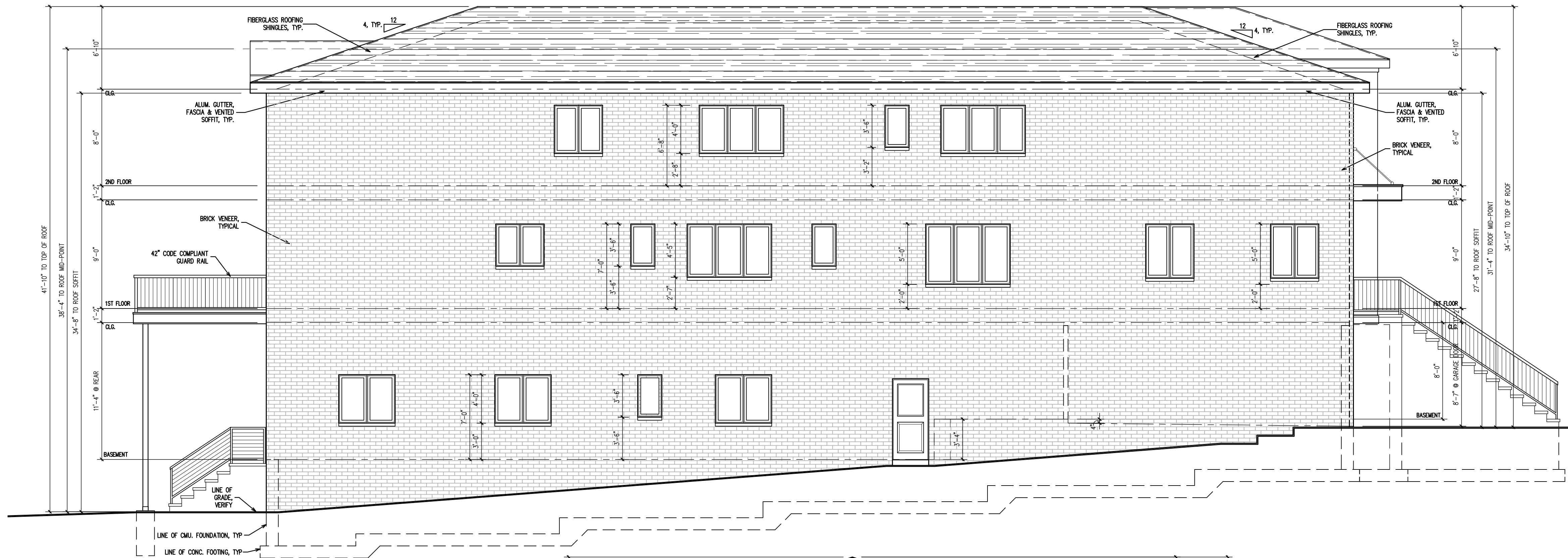
LEFT ELEVATION SCALE: 3/16" = 1'-0" (RIGHT ELEVATION SIMILAR)
