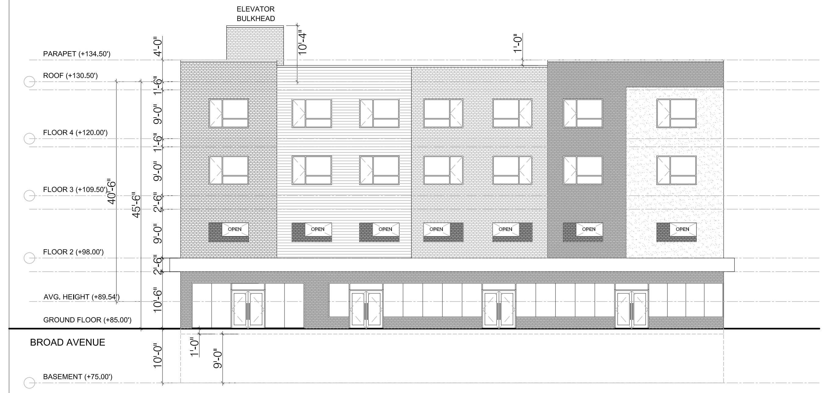
3 PROPOSED REAR ELEVATION SCALE: 3/32"=1'-0"
